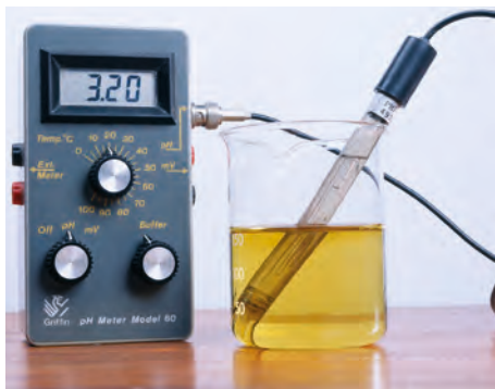
FIGURE 4.3.2 A pH meter is used to measure the acidity of a solution.
