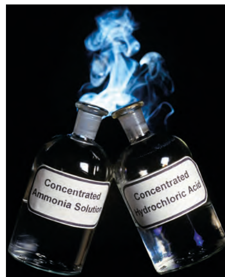
FIGURE 4.1.7 A gaseous acid–base reaction between hydrogen chloride gas and ammonia gas. Fumes of solid ammonium chloride are formed.
